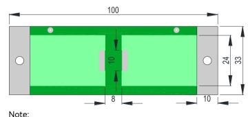
Test Board: 1.6 mm FR4 PCB Copper Thickness: 0.105 mm (3 oz.) for 30 A - 50 A, 0.210 mm (6 oz. ) for 60 A - 125 A
